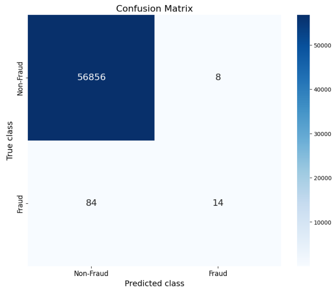
Figure 13: Confusion Matrix of Multilayer Perceptron with Integrated Autoencoder
