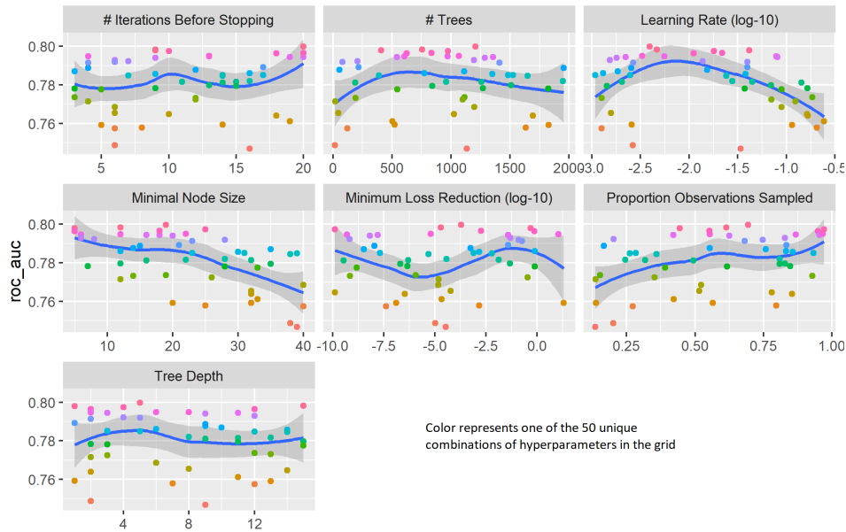
Figure 7: Grid search results for XGBoost. Lines represent locally estimated scatterplot smoothing (loess), and shaded areas around the lines are the 95% confidence intervals.
