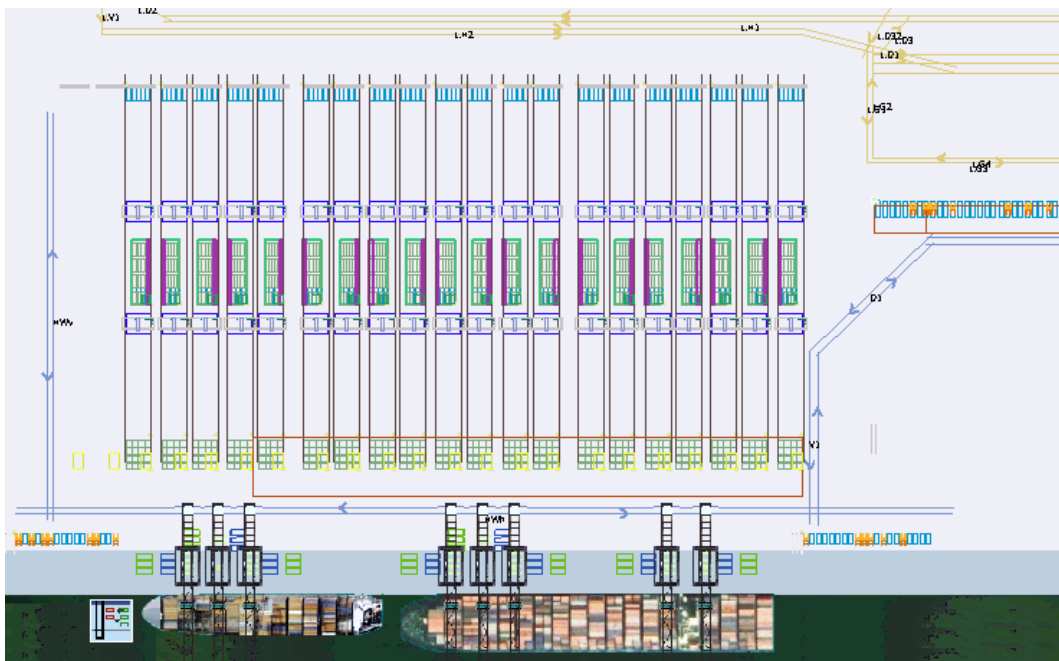
Figure B.3: QC placement CL3 : each of the QCs is placed within two cranywidths of at least one other QC. There are three clusters: two with 3 QCs and one with 2 QCs (Screenshot TBA Simulation model TIMESQUARE).
