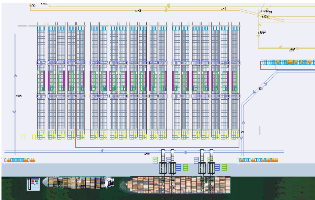
Figure B.4: The off-peak simulated terminal with 4 QCs and a highly decreased throughput (Screenshot TBA Simulation model TIMESQUARE).
