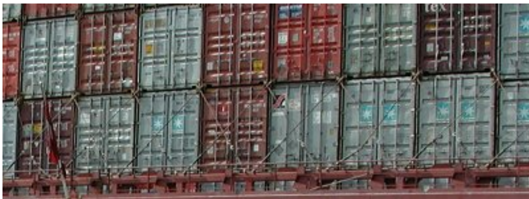
Figure 2.2: Standard containers secured with lashing rods (TBA Training Portal).
