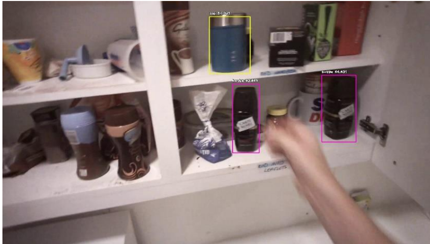
Figure 25 RetinaNet object detection on multiple custom objects. Yellow box = cup, pink box = bottle.
