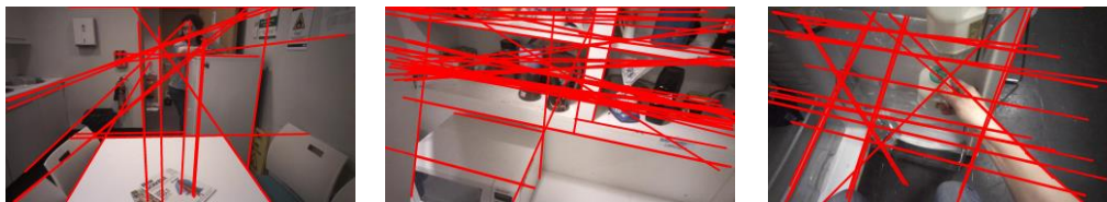
Figure 29 PPHT too much lines detected.
