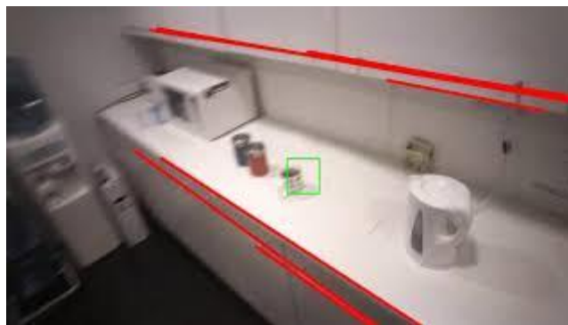
Figure 32 Screenshot from video with detected lines and cups
