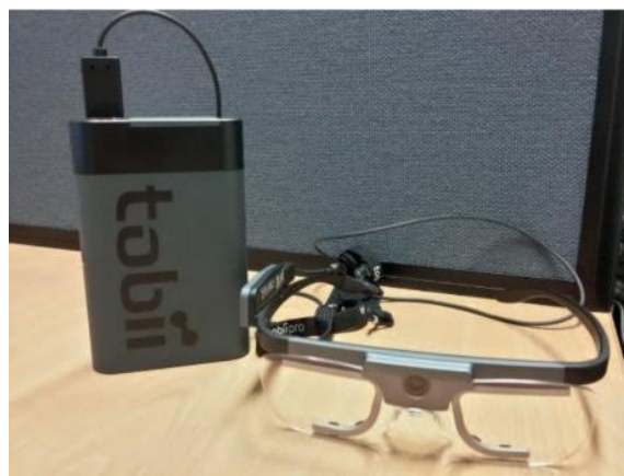
Figure 7 The Tobii 2 glasses system. Reprinted from "The central bias in day-to-day viewing," by F. Ioannidou, F. Hermens & T.L. Hodgson, 2016, Journal of Eye Movement Research , 9, p. 4
