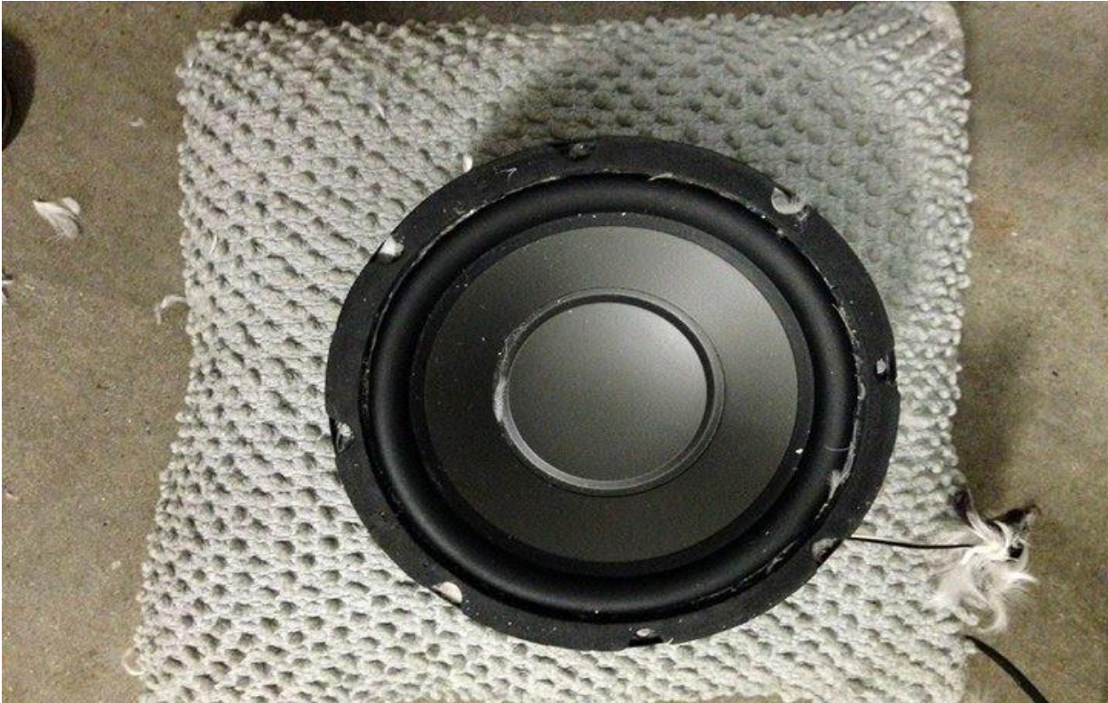
Figure 4. The speaker that was placed inside the pillow to mimic the sound and movement of the heart
