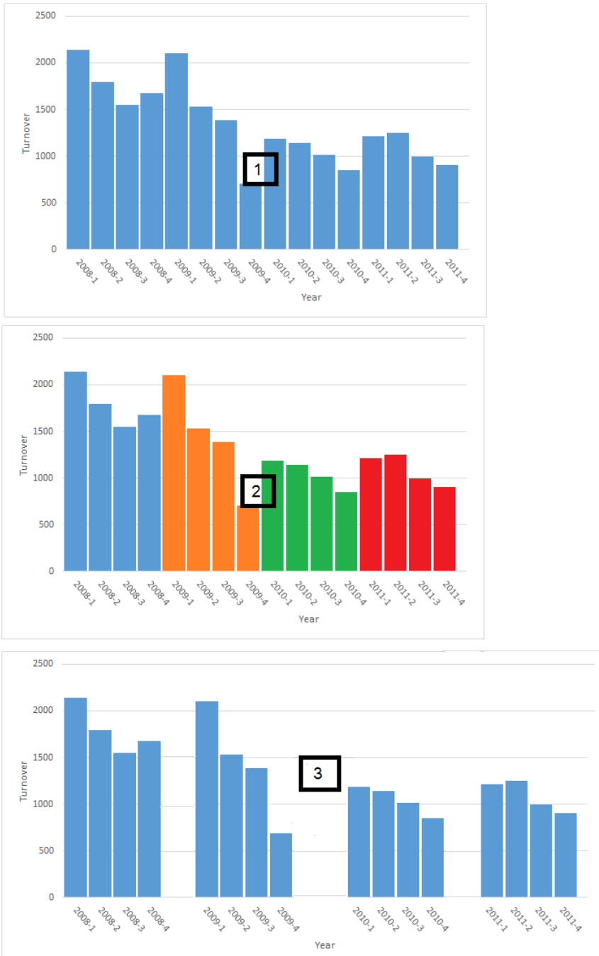
Figure 1.5: An example of lowering the extraneous cognitive load by using the Gestalt principle similarity. In bar chart [1] the bars have the same color and are not separated. The extraneous cognitive load is lowered by chunking the information in bar chart [2] and [3]. The categories are indicated by color [2] or by inserted spaces [3].
